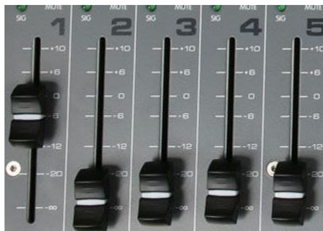
Some faders. The scale on the right is in dB relative to a “unity gain” level near the top (0 dB)
